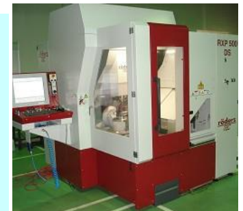
5-axes control machining center by Roeders for die making
